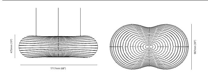
Primary Material Dimensions Fixture Weight Lamp Required Package Dimensions Package Weight Bamboo plywood 1717mm (68") l x 987mm (39") w x 475mm (19") h 3.4kg E27/26 x1 1250mm (49") x 620mm (24") x 50mm (2") 18kg (40lb)
